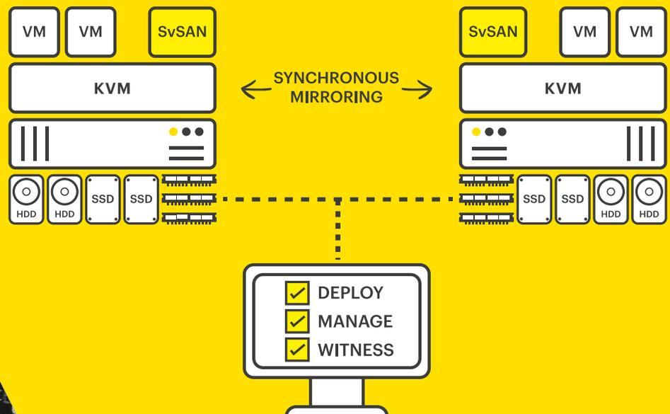
A typical two-node SvSAN configuration
